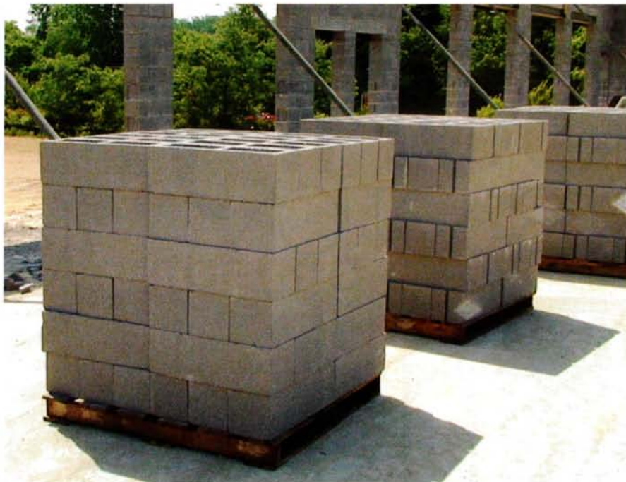
E-Lite lightweight masonry units are comprised of 60% Livlite, 28% natural aggregates, and 12% cement and water. Livlite qualifies as a reclaimed material in applying for LEED credits.
