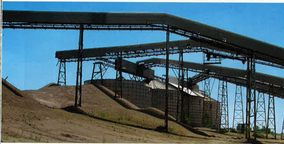
At the Arkalite mine, both silos and open stockpiles are used to store and sort the final product.
